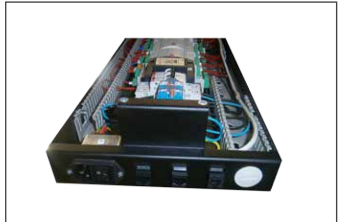
New position of connectors from the bottom of the electro box. Power supply (C14) one-phase with switch, network connectors (RJ45) COM1 and COM2, and service port (RJ12) for service display connection).
