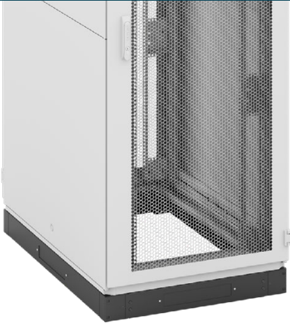
An example of an assembled modular plinth 800 × 1000 mm with a 100 mm height under RF1 rack. Individual parts of the plinth are shown below.
